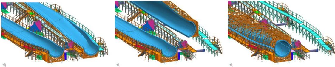
**Figure 5:** Closing process of the main mould
