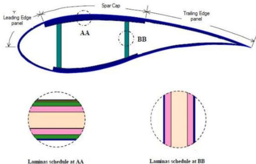
**Figure 1:** Cross section of a composite blade [3]
