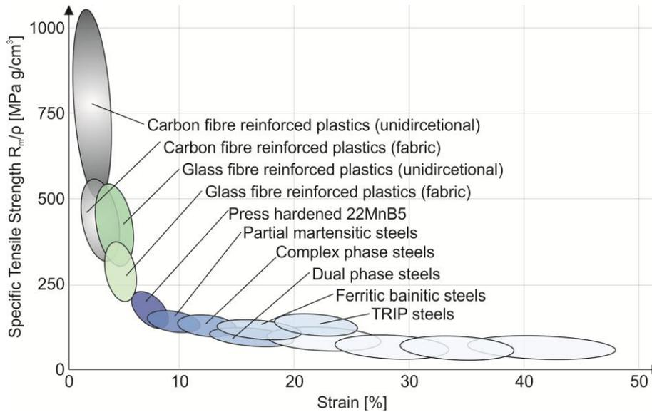
**Figure 2:** Mechanical properties of construction materials
