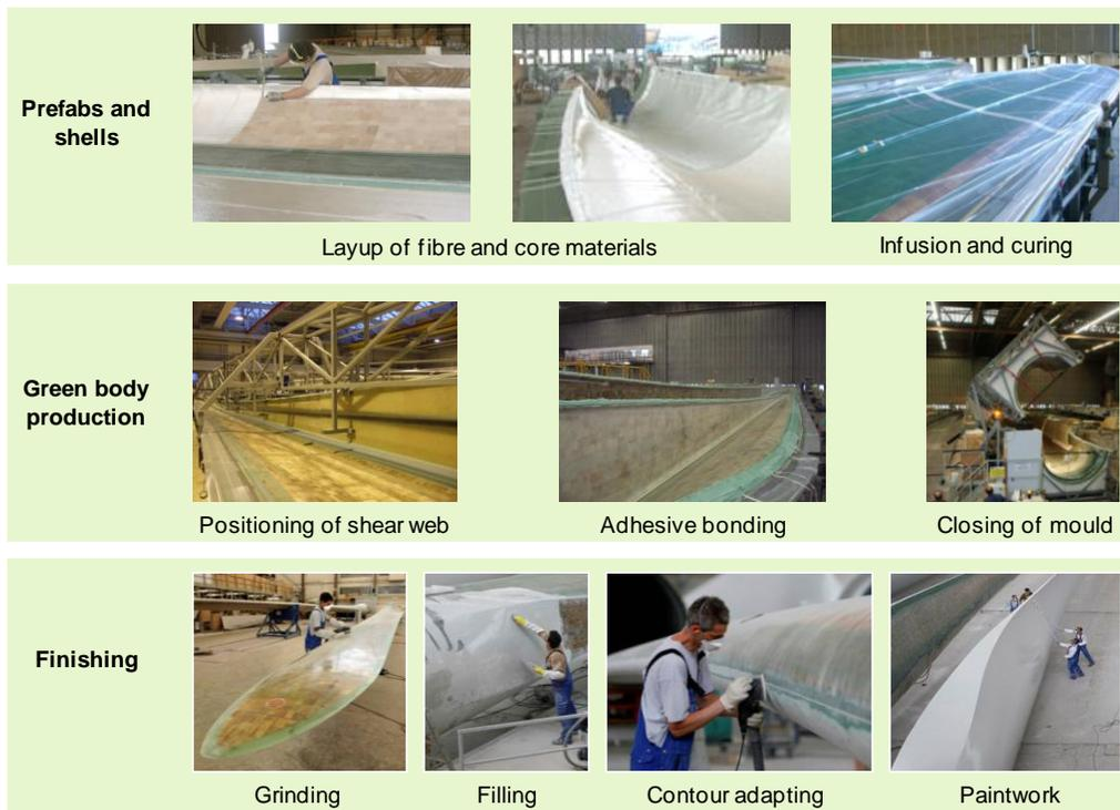
**Figure 6:** Production steps for rotor blades
